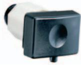
**4112-79 RETROFIT ALL-PURPOSE VALVE** Available for Models B-4063, B-4112, B-2111, B-2112 and B-2014. Field-replaceable corrosion-resistant valve dispenses commercially marketed all-purpose hand soaps. Valve operates with less than 5 lb of force (22.2 N). Patented.
