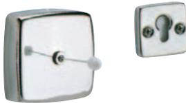
**B-636 SURFACE-MOUNTED RETRACTABLE CLOTHESLINE** Installs over bathtub or in shower. 8-ft (244cm) clothesline pulls out for convenient use; retracts neatly out of way. Retainer bracket mounts on opposite wall to secure clothesline. Cover and retainer bracket are bright polished stainless steel. Unit 3 5/8" x 3 5/8" (90 x 90mm); projects 1 1/4" (30mm) from wall. Av. Mtg. Ht.: 70" (1780mm) to top of unit; Barrier-Free 38–48" (965–1220mm).
